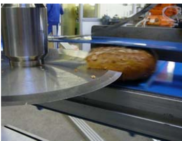
Image: Döinghaus cutting and more Döinghaus will exhibit his new developed rotating ultrasonic round blade in a horizontal cutting machine.
